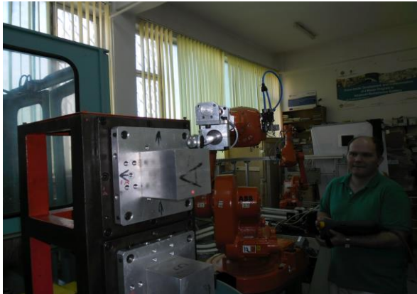
Figure 19. Flexible multi nest prismatic device explored by laser mirror. The problem is that the measurement resolution is modest by about \pm 0.02 and in addition requires the presence of the operator. [2], [4]
