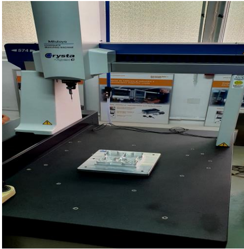
Figure 14. Removable palette with representative part number 1 on the computer measuring machine table.
