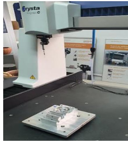
Figure 15. Removable palette with representative part number 2 on the computer measuring machine table.
